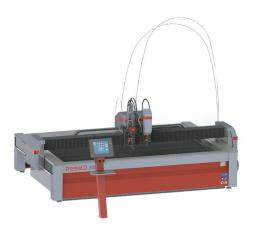
The cutting table comprises a precision-built steel construction embodying linear direct-drive motors on each of the two main axes. To achieve the required precision, the bridge and self-propelled carriage plate are powered by two direct-drive linear motors on each side. This results in a speed range from 1 to 30.000 mm/min.
