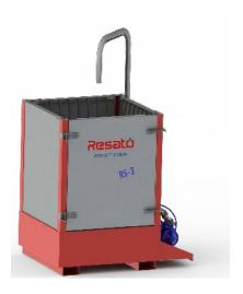
The type RS3 abrasive removal system, containing a single filter, incorporates a special suction and pressure tubing network, provided with a number of inlet and outlet nozzles, that is built into the ACM table's catcher.
