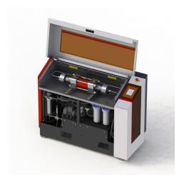
The Resato PJ4-4000 pump works on the pressure booster principle being powered by an electrically-driven hydraulic pump with only 25 liters of oil. The intensifiers pressure is stepless controllable through the HMI or pump from 300 to 3800 bar working pressure. The pump with its touchscreen PLC will follow the instruction of the program and will only consume power and water if required.
