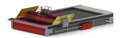
While the table previously was unreachable during cutting, with the Flex-zone it now can freely and safely be loaded and unloaded during the cutting process. Downtime is kept to a minimum while production and operator work-time is optimised.
