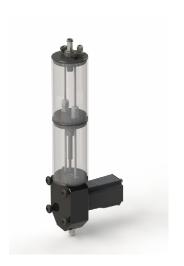
Abrasive costs in general account approximately two-third of total operation costs on a abrasive water jet machine. The abrasive feeder is designed to deliver a dosed amount of abrasive to the waterjet cutting process. It consists of two barrels and a dosing control unit.
